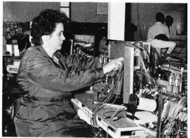
RIGHT: A mains input unit for Myriad being assembled by Mrs. Lilian Francis. This unit distributes power to the sections of the computer. ABOVE: Jack Warner, Foreman, left, with Wilf Chorley who has completed thirty-eight years service
