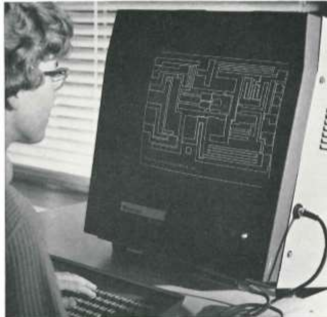
Design of integrated circuit masks using a tracker ball
