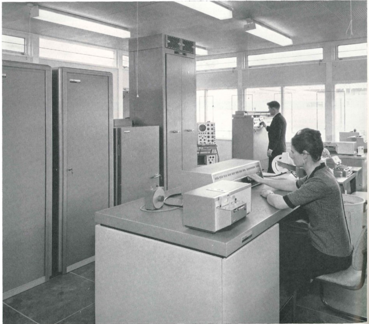
AREA TRAFFIC CONTROL The MYRIAD I computer in the control centre at Glasgow, where the Ministry of Transport's Road Research Laboratory is carrying out an experimental scheme
